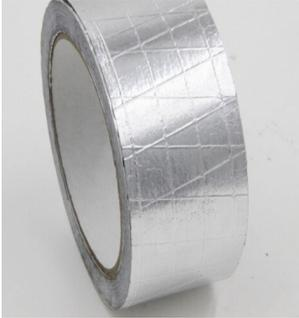
\* Fiberglass Reinforced Aluminum Foil Tape GF0301-212 is coated with hot melt adhesive on dead soft aluminum foil with different thicknesses. It is excellent for sealing joints, seaming against moisture and vapor on foil jacketing insulation, etc.
